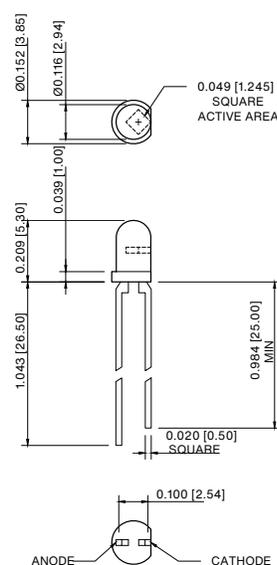
Lead soldering temperature (3mm from body) 260 $^\circ\text{C}$  for 5 sec.
