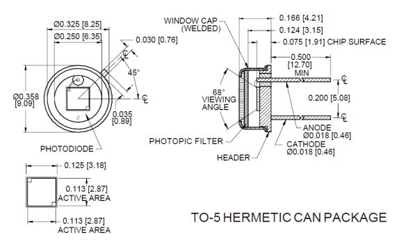
> Soldering Conditions: 260°C 1/16 inch away from case for 3 seconds max.
