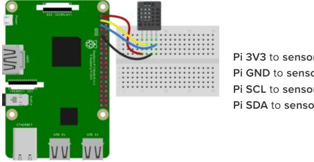
Pi 3V3 to sensor VIN Pi GND to sensor GND Pi SCL to sensor SCL Pi SDA to sensor SDA
