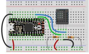
Board 3V to sensor VIN Board GND to sensor GND Board SCL to sensor SCL Board SDA to sensor SDA
