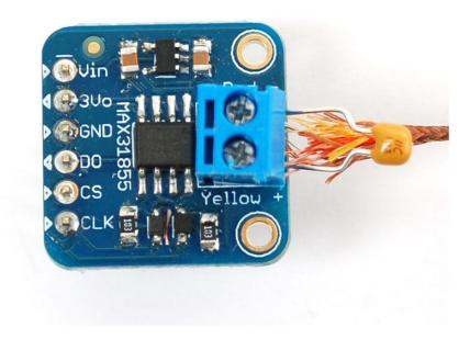
If you are using the MAX31855 v1.0 in a noisy environment, you may need to add a 0.01uF capacitor across the thermocouple leads.
