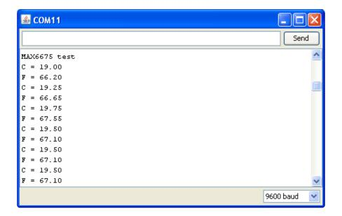
As you can see, its pretty simple to use the library, simply tell the sensor object what the clock, chip select and data pins are, then call **readCelsius()** or **readFahrenheit()** to get a floating point result.
