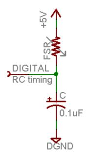
In this case, our 'bucket' is a 0.1µF ceramic capacitor. You can change the capacitor nearly any way you want but the timing values will also change. 0.1µF seems to be an OK place to start for these FSRs.
