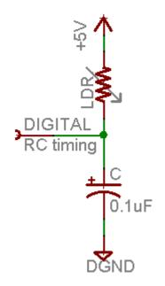
In this case, our 'bucket' is a 0.1uF ceramic capacitor. You can change the capacitor nearly any way you want but the timing values will also change. 0.1uF seems to be an OK place to start for these photocells. If you want to measure brighter ranges, use a 1uF capacitor. If you want to measure darker ranges, go down to 0.01uF.
