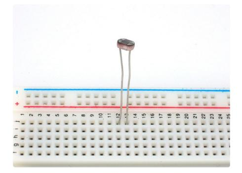
Photocells are pretty hardy, you can easily solder to them, clip the leads, plug them into breadboards, use alligator clips, etc. The only care you should take is to avoid bending the leads right at the epoxied sensor, as they could break off if flexed too often.
