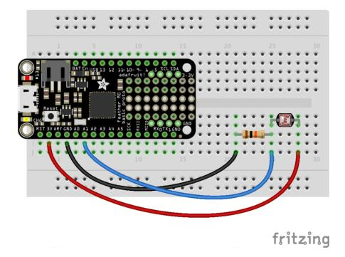
Here's an example of wiring a photocell to a Feather MO:
