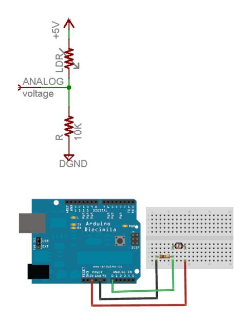
For this example I'm showing it with a 5V supply but note that you can use this with a 3.3v supply just as easily. In this configuration the analog voltage reading ranges from 0V (ground) to about 5V (or about the same as the power supply voltage).
