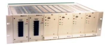
The OLC53 Series of AC/DC converters uses high frequency half-bridge topology to generate 200W output power. Virtually any DC output is possible with short delivery times. This low profile design features low component count and high efficiency. The use of professional quality components and rigorous quality control results in an MTBF exceeding 100,000 hours at 45°C.
