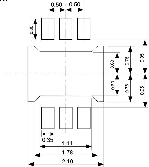
Caution It is recommended to solder the heat sink to a board in order to ensure the heat radiation.
