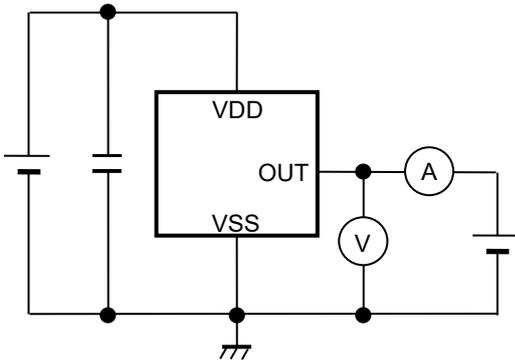
**Figure 8 Test Circuit 3**
