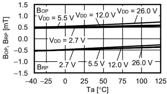
**2.6.2 Operation point, release point ( $B_{OP}$ ,  $B_{RP}$ ) vs. Power supply voltage ( $V_{DD}$ )**
