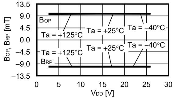
**Caution**  $V_{DD} = 2.7\text{ V to }5.5\text{ V}$  when output form is Nch driver + built-in pull-up resistor (1.2 kΩ typ.).
