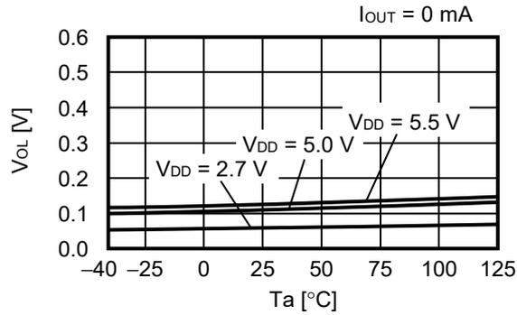
1.3.2 Low level output voltage ( $V_{OL}$ ) vs. Power supply voltage ( $V_{DD}$ )
