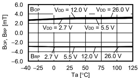
**2.8.2 Operation point, release point ( $B_{OP}$ ,  $B_{RP}$ ) vs. Power supply voltage ( $V_{DD}$ )**
