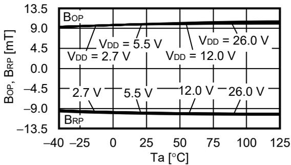
**2.10.2 Operation point, release point ( $B_{OP}$ ,  $B_{RP}$ ) vs. Power supply voltage ( $V_{DD}$ )**
