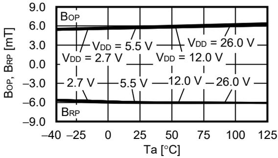
**2.9.2 Operation point, release point ( $B_{OP}$ ,  $B_{RP}$ ) vs. Power supply voltage ( $V_{DD}$ )**
