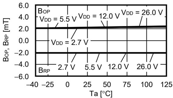
**2.7.2 Operation point, release point ( $B_{OP}$ ,  $B_{RP}$ ) vs. Power supply voltage ( $V_{DD}$ )**
