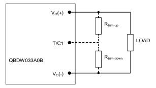
Figure 16. Circuit Configuration to Trim Output Voltage.
