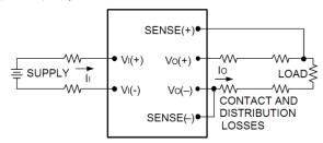
Figure 15. Circuit Configuration for remote sense.
