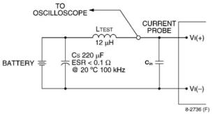
Note: Measure input reflected-ripple current with a simulated source inductance (LTEST) of 12  $\mu$ H. Capacitor CS offsets possible battery impedance. Measure current as shown above.
