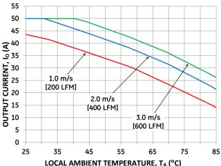
Figure 19. Output Current Denating for the Base plate QSD(V)W050A0B-H with Longitudinal Airflow from Vout to Vin; Vin=48V.
