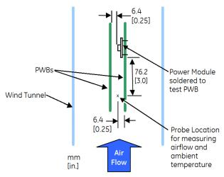
The power modules operate in a variety of thermal environments and sufficient cooling should be provided to help ensure reliable operation. Thermal considerations include ambient temperature, airflow, module power dissipation, and the need for increased reliability. A reduction in the operating temperature of the module will result in an increase in reliability.
