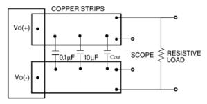
Note: Use a Cout  $\,(470~\mu F$  Low ESR aluminum or tantalum capacitor typical), a  $0.1~\mu F$  ceramic capacitor and a  $10~\mu F$  ceramic capacitor, and Scope measurement should be made using a BNC socket. Position the load between 51 mm and 76 mm (2 in. and 3 in.) from the module.
