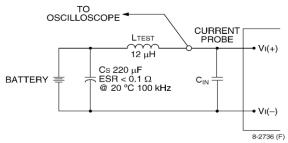
Note: Measure the input reflected-ripple current with a simulated source inductance (LTEST) of 12  $\mu\text{H}.$  Capacitor CS offsets possible battery impedance. Measure the current, as shown above.
