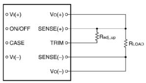
Figure 14. Circuit Configuration to Increase Output Voltage.
