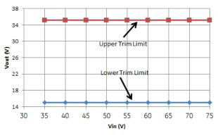
Figure 12. Output Voltage Trim Limits vs. Input Voltage.
