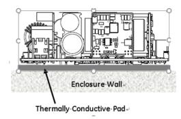
Note that the Ambient Temperature shown in Table 1 is that outside the sealed enclosure, the unit may see higher ambient temperatures.
