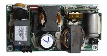
In a small 2 x 4-inch footprint, the 48Vdc or 54Vdc single-output CLP0248 open frame power supply delivers greater than 88 percent typical power efficiency at 25°C and full load output at +50°C. With its small size, the CLP series is specifically designed to handle power challenges associated with tight space and low airflow.
