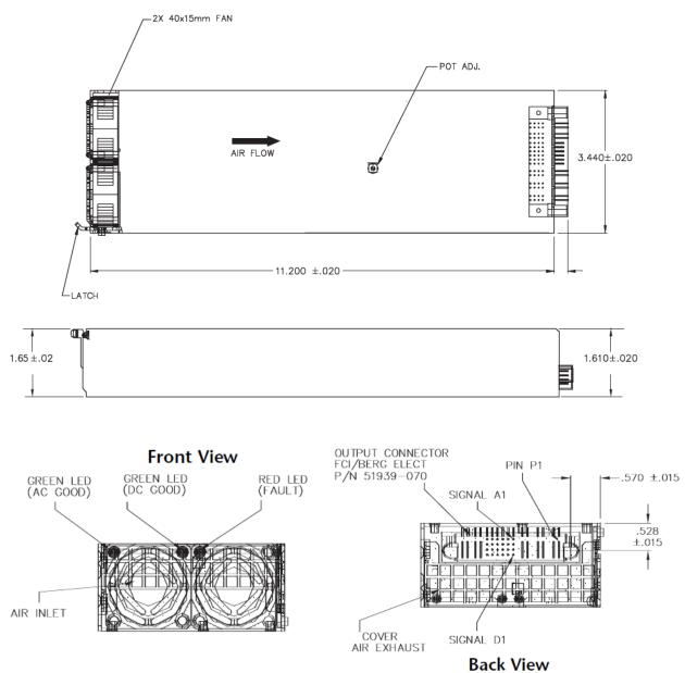
Input: 90Vac to 264Vac; Output: -54Vdc @ 1200W
