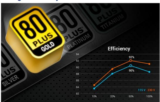
The Dagger Series is 80 PLUS Gold certified power supply units that guarantee to operate at a minimum of 90% efficiency at 50% load of PSU rated power which has lower running costs with less electrical waste.
